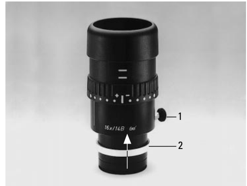
Fig. 93 Eyepiece 16x/14B 1 Clamp screw, 2 Spacer rings for Leica microscopes (must be pushed up as far as the stop)
